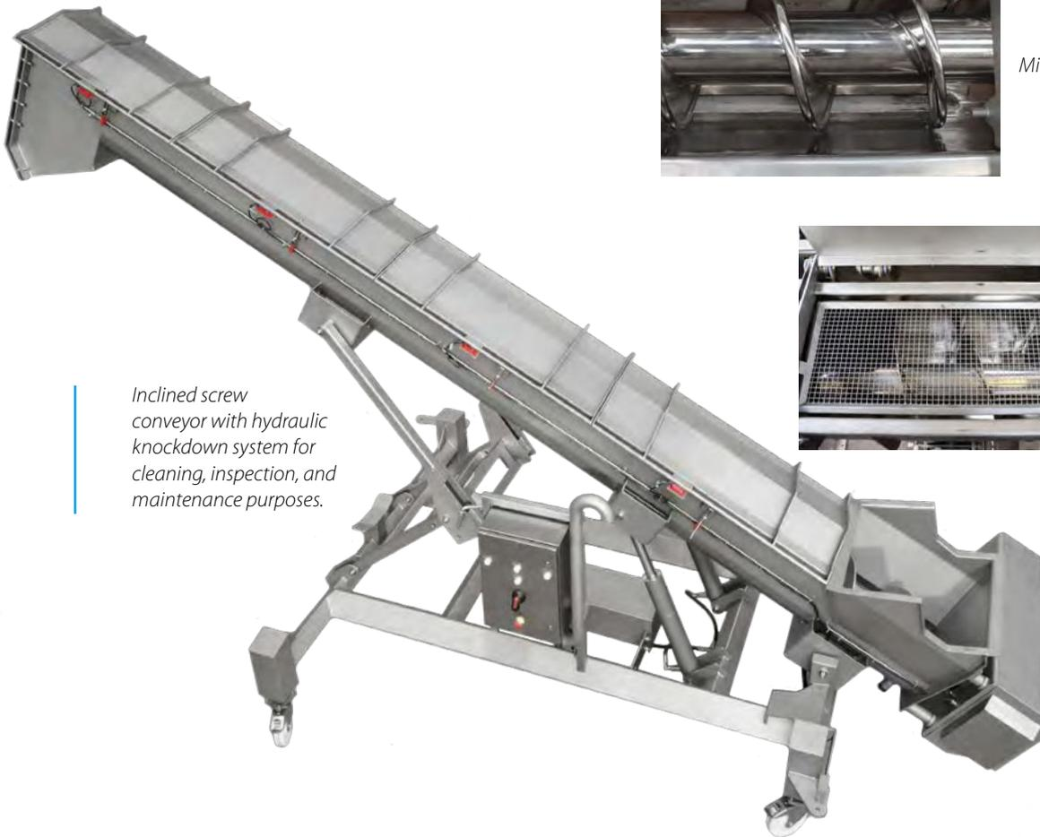
*Inclined screw conveyor with hydraulic knockdown system for cleaning, inspection, and maintenance purposes.*
