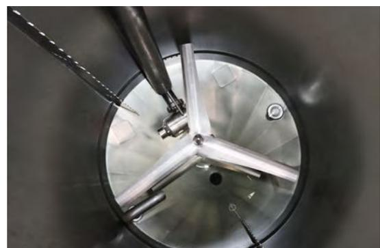
*Mixing container designed for heavy viscous gravies/mixtures. The Ytron and the Venturi system in combination with the Heavy Duty mixing agitators ensure a fast processing of a gravy free from lumps. Anti-vortex breakers are standard in all scanGravy mixing tanks. Direct steam injection for temperature control can be added as well.*
