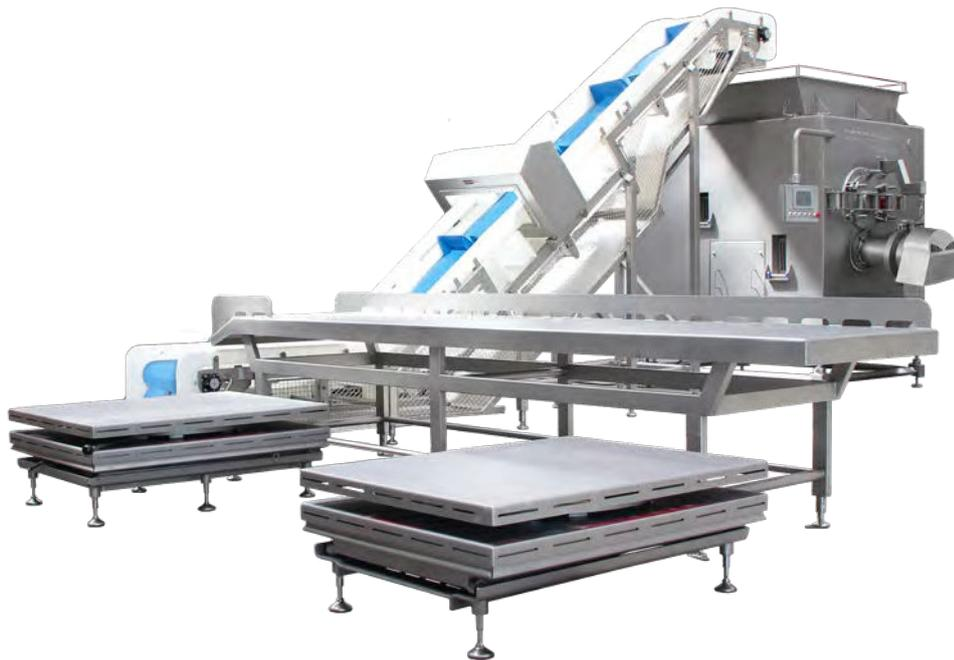
*Example of scansteel foodtech® infeed systems shown with belt conveyor, unpacking station and CombiGrind CG 300 HD*
