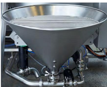
scansteel foodtech® high speed dry ingredients addition Venturi system. For addition of all kinds of dry ingredients. Prevents air injection into gravy during production of same.
