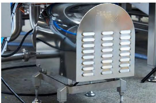
*Pumps are positioned/mounted on their own frame for easy access at inspection/maintenance, etc. In addition, the pump of the scanGravy mixing unit can be equipped with its own knife system for eliminating lumps in "challenging to produce" gravies.*
