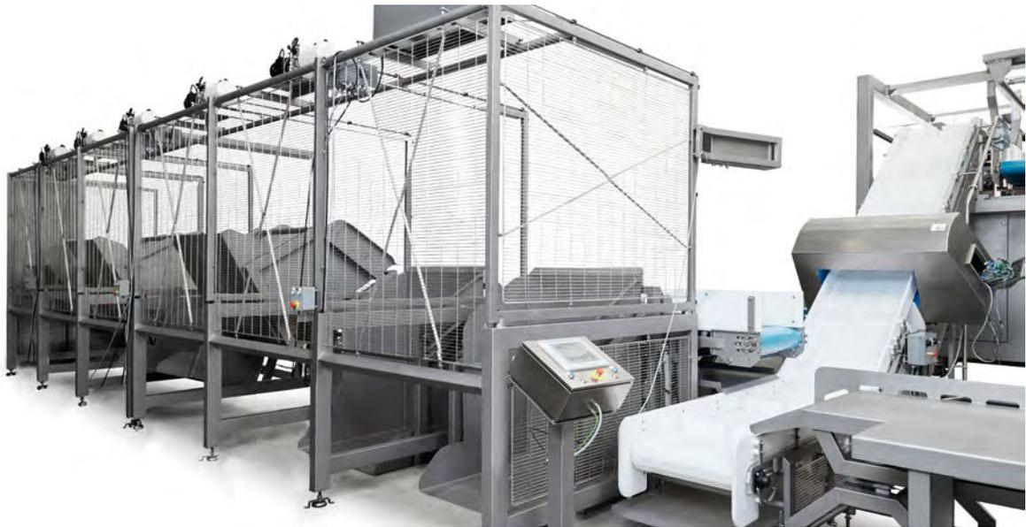
6 (six) unit weighing station, seen from the infeed side. Typically, Dolav bins are fed into the swing loaders by a fork lift truck. All is controllable from the operator panel.
