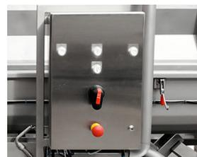
Standard screw conveyor electrical/operator panel.
