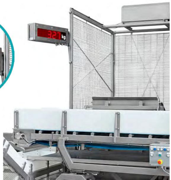
Details showing drip trays and weighing/load cells.
