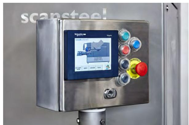
Operator control with easy-to-understand push button operation of start, stop, and emergency. Pre-setting of worm/auger speeds and programming functions with logically designed graphics on the touch panel. Programmes with fixed settings for various products can be keyed in with password protection. The scansteel foodtech® scanControl function can be set to optimize the feeding worm/auger speed in relation to the grinding worm/auger, thus reducing grinding capacity flow fluctuations.
