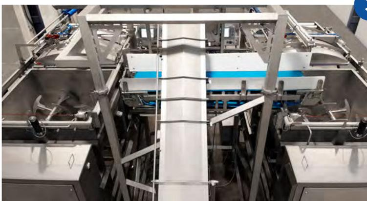
Close-up view showing scansteel foodtech® inclined screw conveyor feeding onto a scansteel foodtech® horizontal belt conveyor which has 3 (three) main positions.
