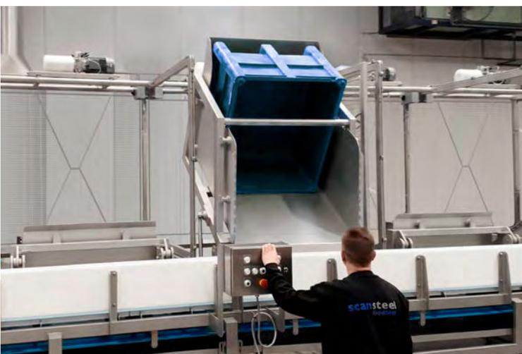
With the scansteel foodtech® line control, it is possible to guide the operator into the exact amount of each meat raw material to be unloaded onto the weighing/batching belt conveyor.
