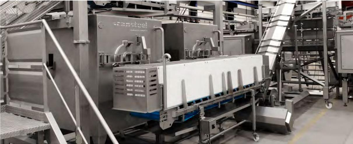
Another typical horizontal belt conveyor solution where 2 (two) grinders are discharging onto the scansteel foodtech® belt conveyor. This solution saves a lot of safety devices and, at the same time, secures easy access to the grinders for cleaning, mounting, and dismounting of the grinders, front view.
