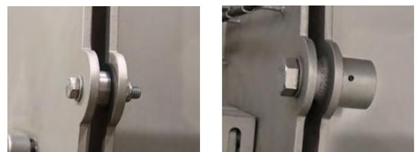
View of standard bolt system and safety bolt system.
