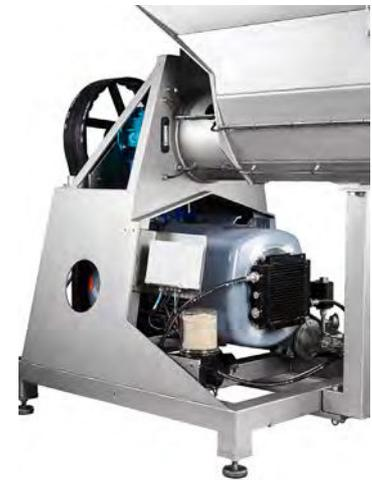
SuperGrind 400/260 shown with all side panels dismantled, side view. Designed for easy access at maintenance and inspection. The automatic greasing system for main bearing and front bearing is also shown.
