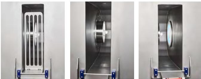
Hygienic zone shown in 3 (three) positions: running position (closed) and cleaning position shown from both angles.
