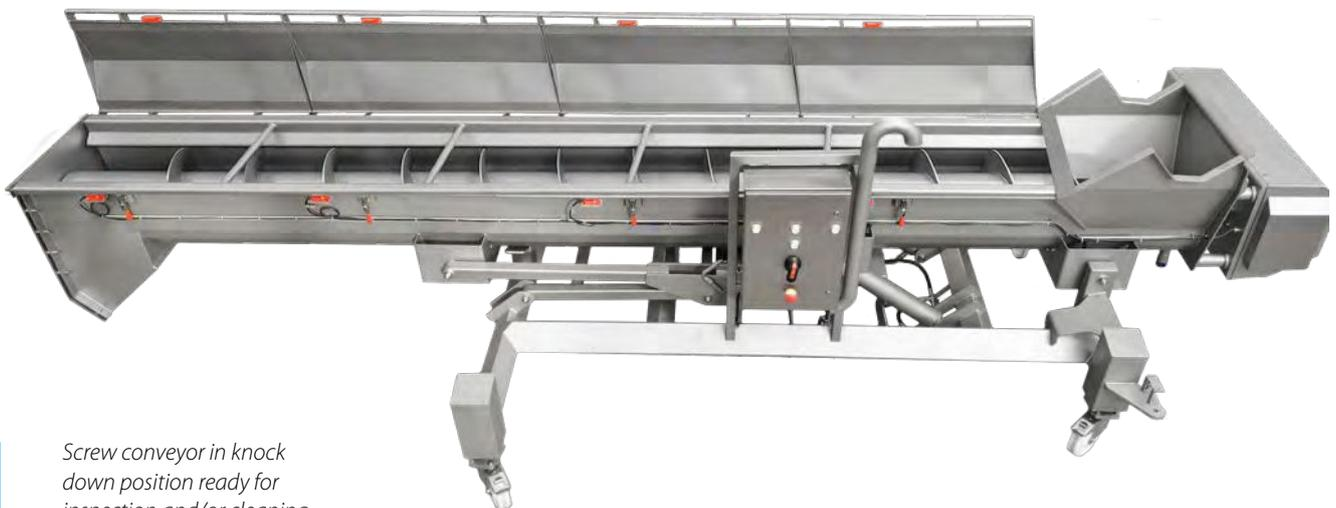
*Screw conveyor in knock down position ready for inspection and/or cleaning.*
