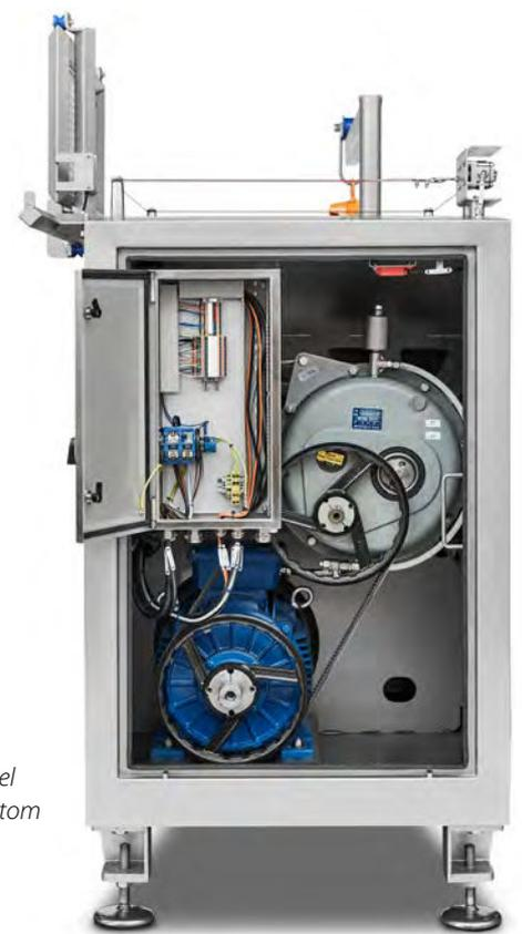
*MG 200 shown with back panel open. All stainless steel construction, including bottom frame.*
