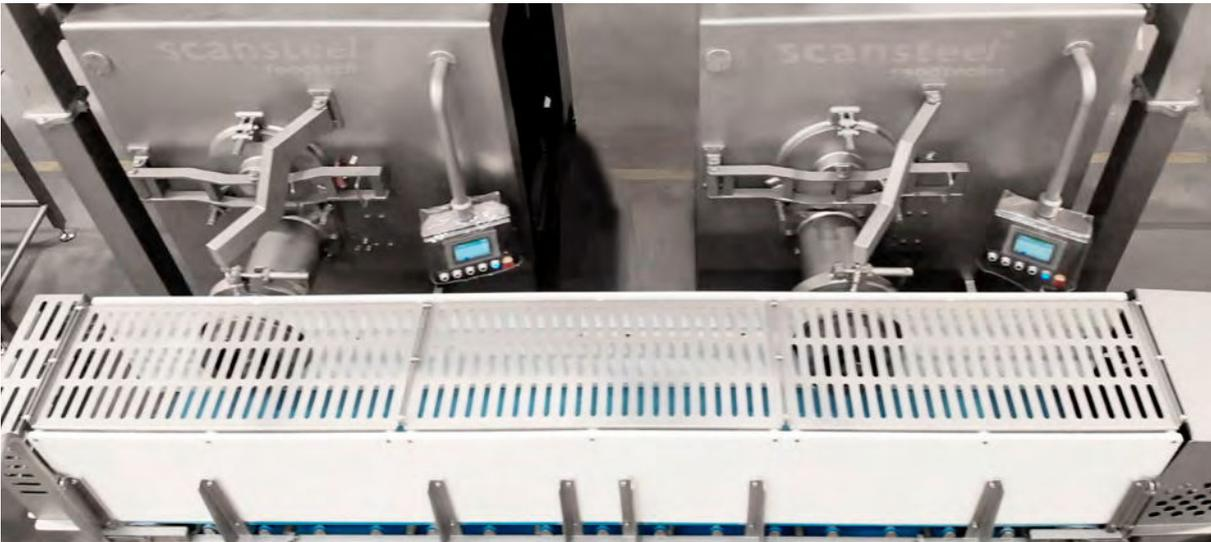
Another typical horizontal belt conveyor solution where two grinders are discharging onto the scansteel foodtech® belt conveyor. This solution saves a lot of safety devices and, at the same time, secures easy access to the grinders for cleaning, mounting and dismounting of the grinders, top view where the transfer point from grinders to belt conveyor is clearly seen.
