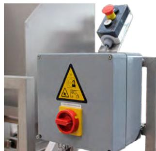
Operator/control panel with emergency stop.
