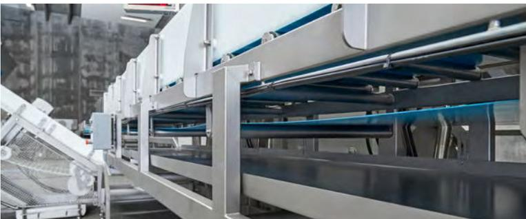
All scansteel foodtech® belt conveyors can upon customers request be manufactured with drip trays/ collection pans in order to avoid moisture on the floor.
