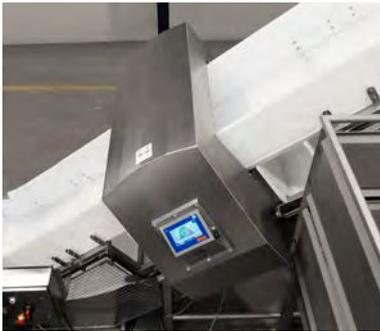
*Standard scansteel foodtech® inclined belt conveyor with metal detector, side view. scansteel foodtech A/S can deliver our belt conveyors with any brand type metal detector. Side view.*
