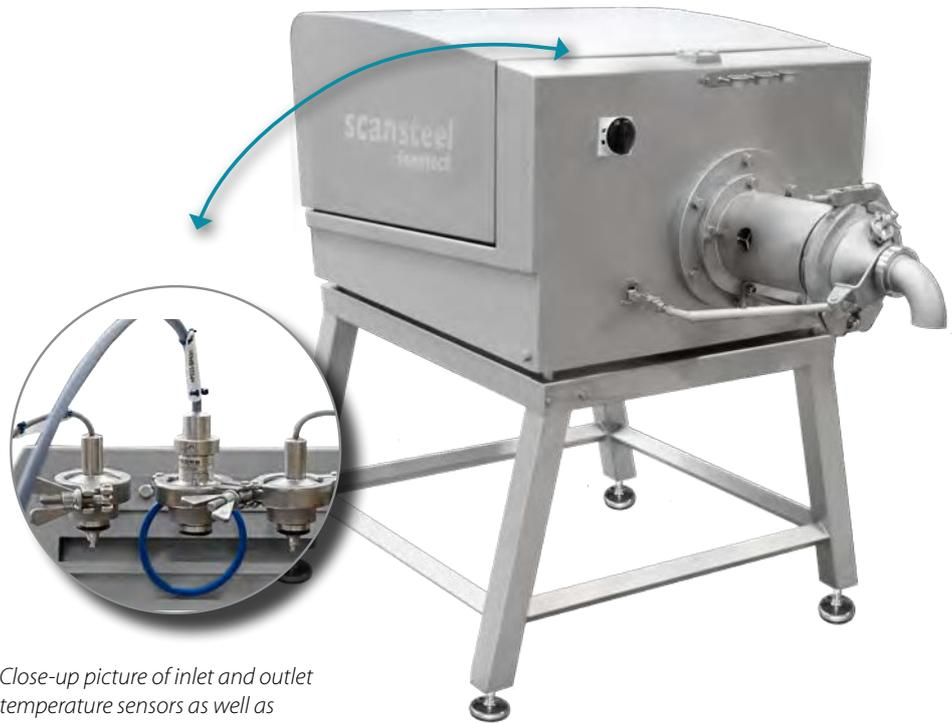
Close-up picture of inlet and outlet temperature sensors as well as pressure transducers.
