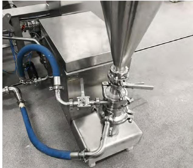
The mixing tank is used to dissolve or disperse powdered products in a liquid or to mix different liquids, with the Ytron powder dispenser for dissolving all dry "challenging to add" matters/ingredients in the gravy and/or the brine.
