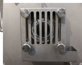
View of the silo discharge screw bearing with and without safety cover.
