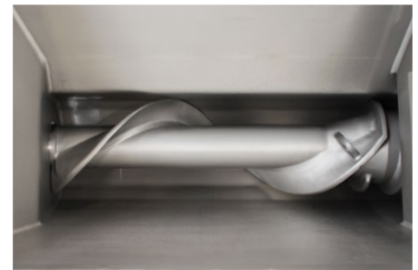
Infeed hopper shown from top view. Please note the grinding worm/auger with the sharp knife edge, designed to grab and feed both frozen blocks and fresh meat raw materials.
