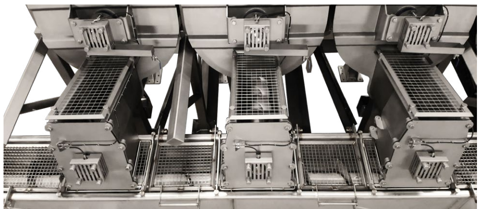
View of the silo discharge screw bearing with and without safety cover.
