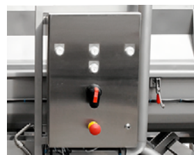
Standard screw conveyor electrical/operator panel.
