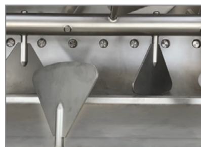
Paddle mixing wings, special application.
