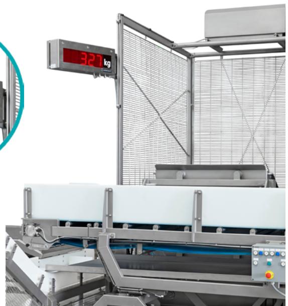
Details showing drip trays and weighing/load cells.
