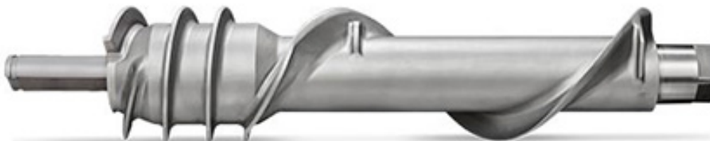
Heavy Duty designed worm/auger with sharp knife edge on hopper part of worm/auger to grab frozen blocks.
