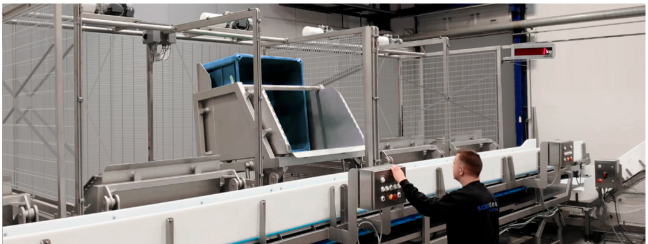
One option in the scansteel foodtech® "batching family of solutions" is a station of typically 2 – 8 swing loaders (tippers) which can hold different meat raw material.
