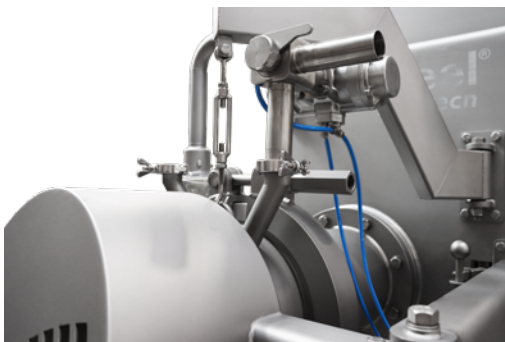
A prime example of scansteel foodtech® hygienic design is given by the hygienic zone positioned between the worm/auger and the gear box. Hygienic zone shown in running position (closed) and in cleaning/inspection position. When opened, the grinder cannot be started until the guard has been positioned in closed position.
