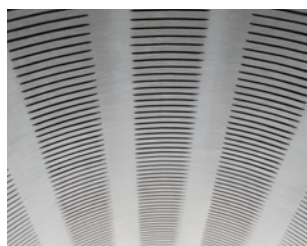
Slit filter seen from inside.
