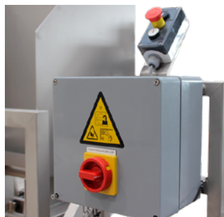
Operator/control panel with emergency stop.
