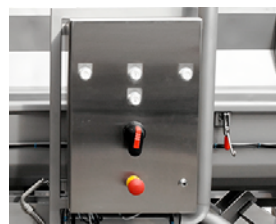
Standard screw conveyor electrical/operator panel.
