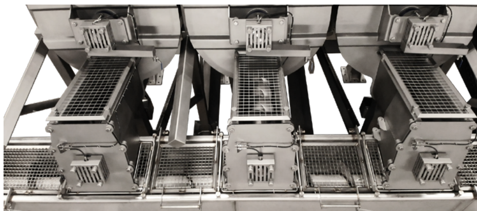
View of the silo discharge screw bearing with and without safety cover.
