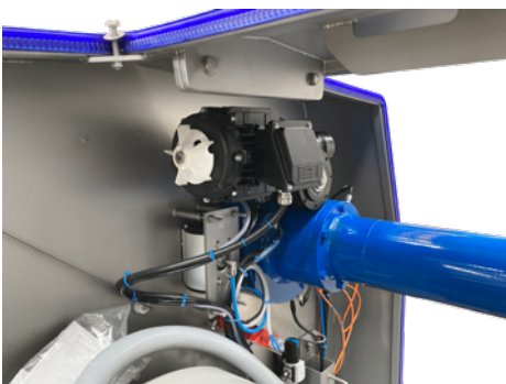
Inside view of QuadroCut 225 output shaft from the left angle.
