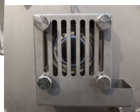
View of the silo discharge screw bearing with and without safety cover.
